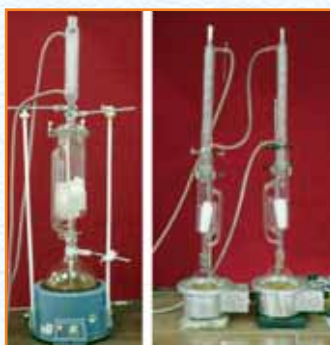
Oil extraction units for direct & indirect methods of oil extraction
