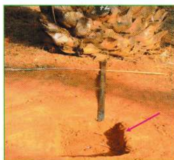
Soil sampling pit point (one metre away from palm base)
