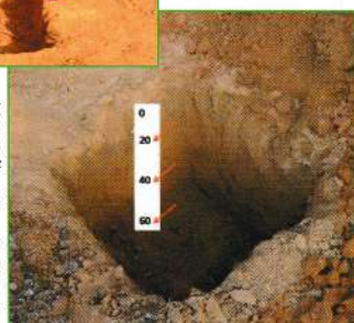
Soil sampling pit point (one metre away from palm base)
